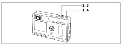
1 Press the power switch for more than 2 seconds.
